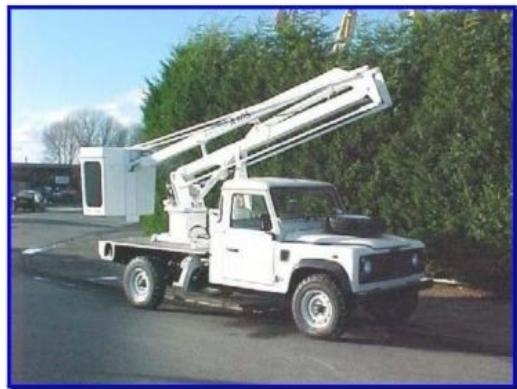
▲ Fully hydraulic controls enable the operator to position the work platform into the optimum position, giving more efficient and safe working conditions.
