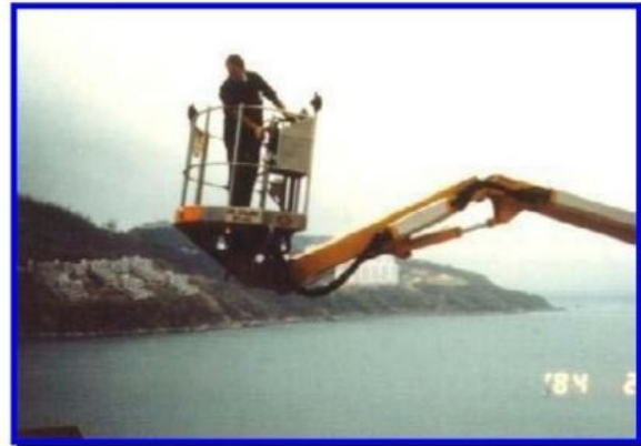
Large (2.21m 2 ) high strength tubular alloy cage with full hydraulic controls, safety belt anchorage, work light, 24v electric take off point
