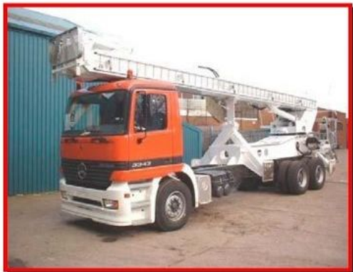
SF280 on Mercedes 3343 ready for custom fire engineering bodywork and fixed pump installation
