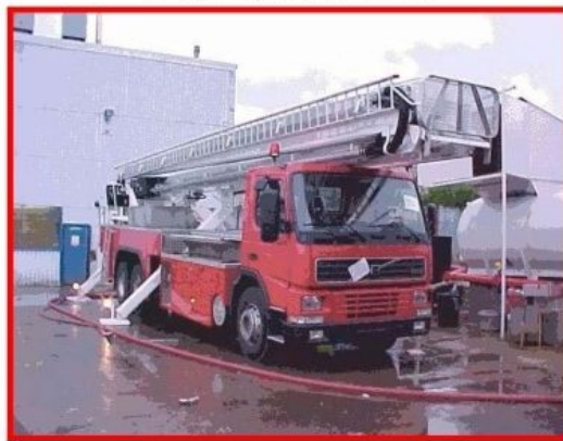
Third boom allows "up and over" feature giving full flexibility to fire-fighters in stressful operations
