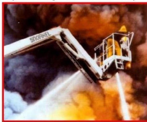
Large high strength tubular alloy cage with full hydraulic controls located at cage front, spot light, 24v electric take off point, water monitor and water hose connection(s)
