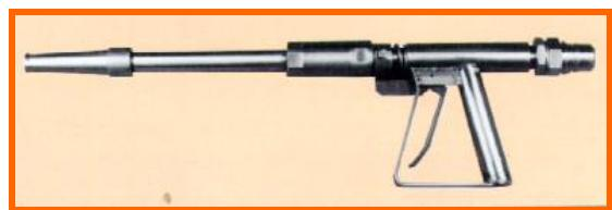
High-pressure stainless steel wash guns with 'dead man' type trigger control, QRC, flow straightener and 1/4 inch nozzle. For high wind conditions, wash guns with 5/16 inch nozzles are available. Pressure gauge and 3m fly hose are optional. All parts interchangeable.
