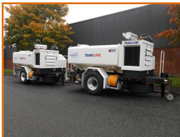
**THE CHANCE LIVE LINE INSULATOR WASHER TRAILER MOUNT SERIES** is fitted to a heavy duty, rugged, rough terrain axle with sand tyres as standard.
