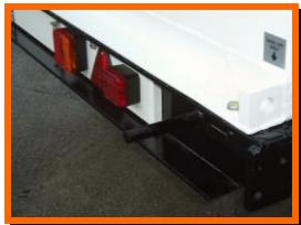
Standard highway lighting package with brakes; indicators and hazard warning.
