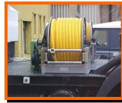
Optional electric rewind hose-reel (50m) with quick release connectors and hose guide.
