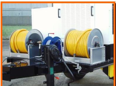
2 manual rewind hose reels with 50m of 1" insulated heavy duty wash hose are fitted as standard (electric rewind optional)
