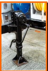
Standard heavy duty adjustable hitch jack to allow easy parking without towing vehicle.
