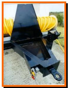
Standard lockable tool compartment for wash gun storage with quick air connectors and tow eye
